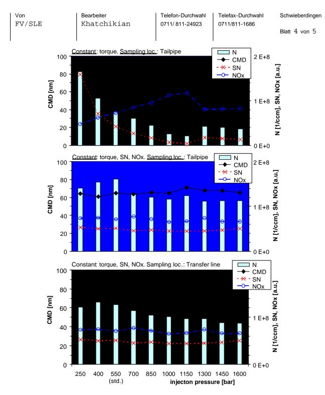
Fig. 1: Particle size (CMD), number concentration (N), smoke number
