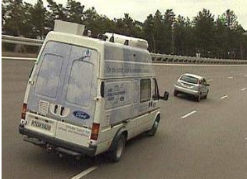
Fig. 4. Chasing of exhaust plume with Ford Mobile Laboratory
